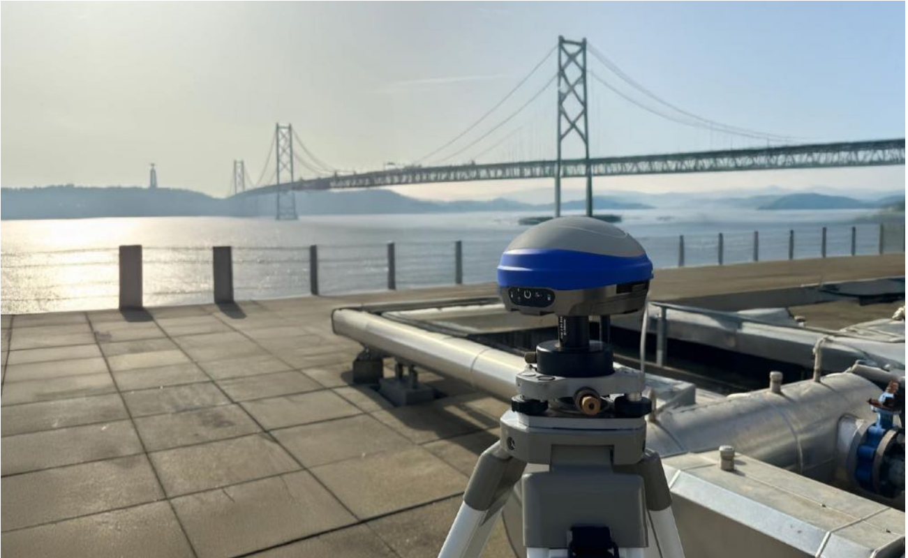
Figure 12 - Viking installed on a tribrach.
