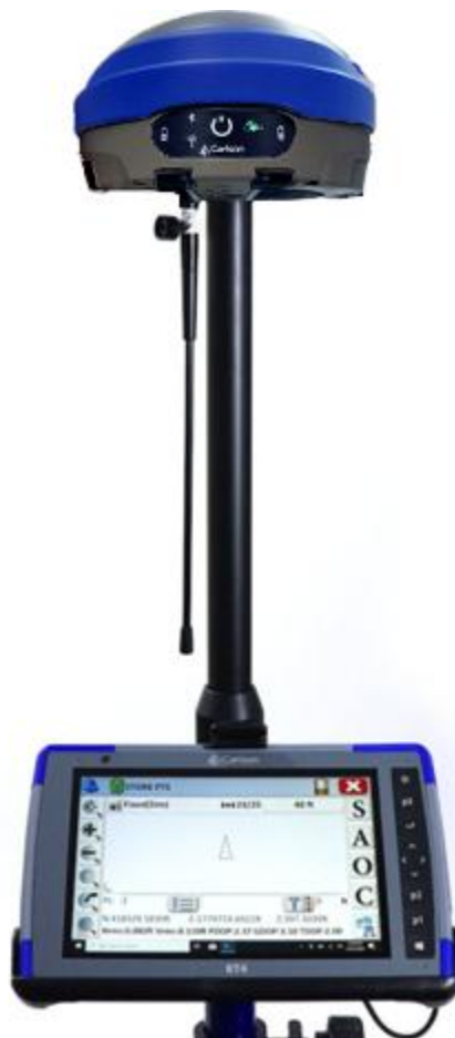
Figure 11 - Viking Installed on range pole with UHF antenna.
